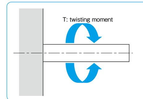
Figure B-5 Deformation of Spline Shaft by Twisting Moment
