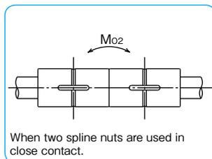
When two spline nuts are used in close contact.
