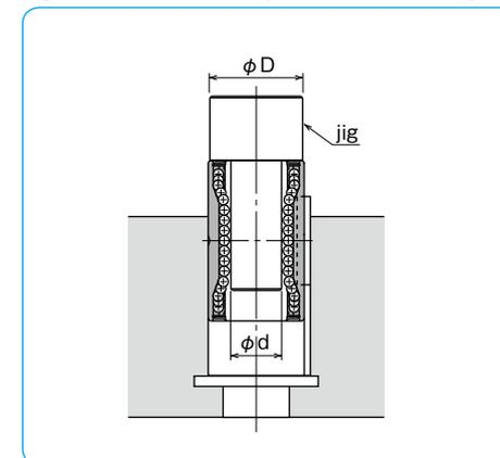
Table B-14 Recommended Jig Dimensions unit : mm
