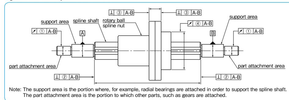
Note: The support area is the portion where, for example, radial bearings are attached in order to support the spline shaft. The part attachment area is the portion to which other parts, such as gears are attached.
