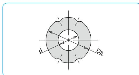
Figure B-11 Example of Shaft-end Machining
