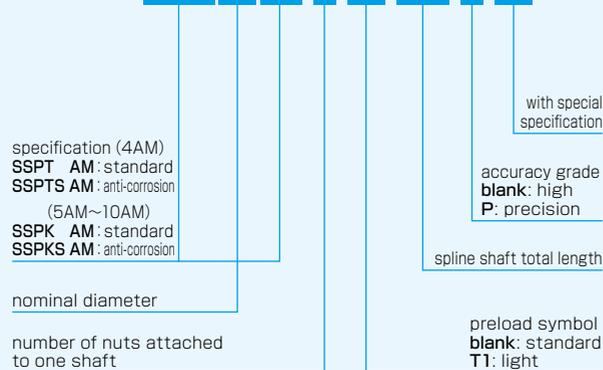
Note: Nut material of SSPT-AM and SSPK-AM is stainless steel.
