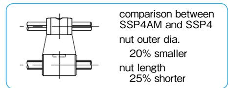
Figure B-1 Basic Structure of NB Ball Spline
