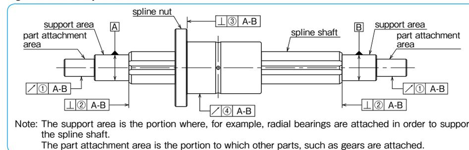
Tolerance of Spline Shaft Groove Torsion (Max.)
