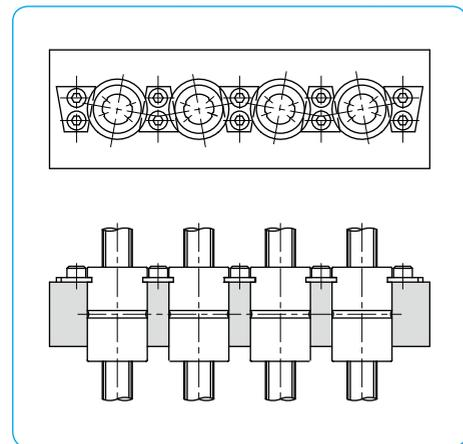
Figure B-23 Using Special Lock Plates (2)
